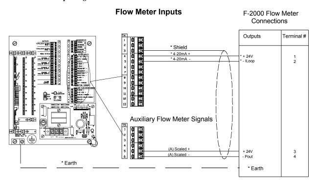
Connections shown with \* are required for all installations. Connections shown with (A) are optional.
