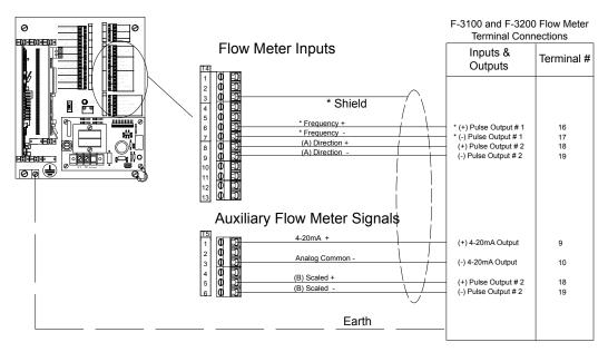
NOTE: The System-10 does not provide power to the F-3100 or F-3200 flow meter. Input power for the flow meter must be provided separately. See flow meter manual for detailed wiring instructions.
