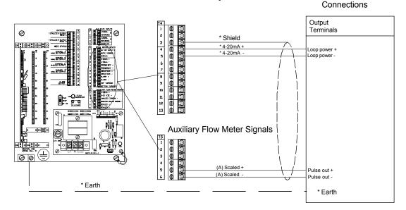
Connections shown with \* are required for all installations. Connections shown with (A) are optional.
