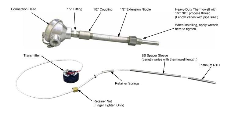
The thermowell, extension nipple, coupling and fitting were made to a specific length. DO NOT attempt to change the length of this assembly.
