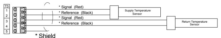
**Insertion Turbine Flow Meter Input Connections**
