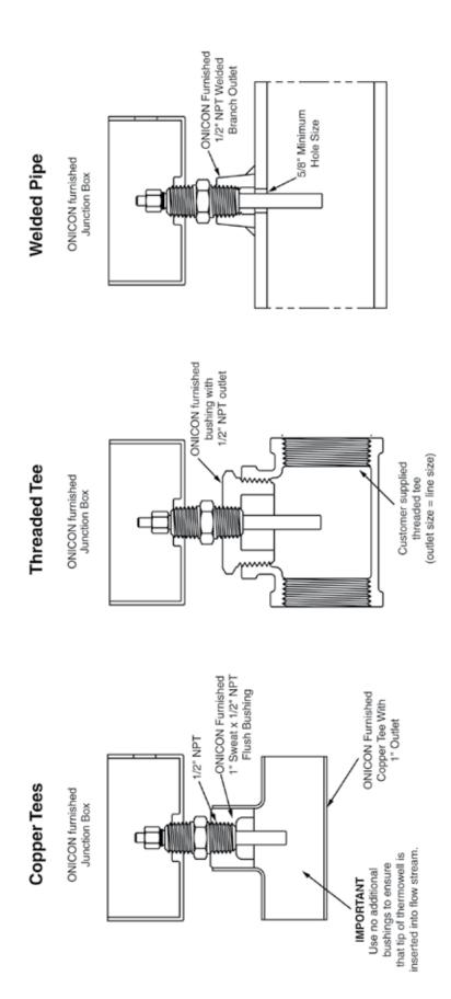
NOTES: 1. If additional fittings are required, ensure that tip of thermowell remains in flow stream.
