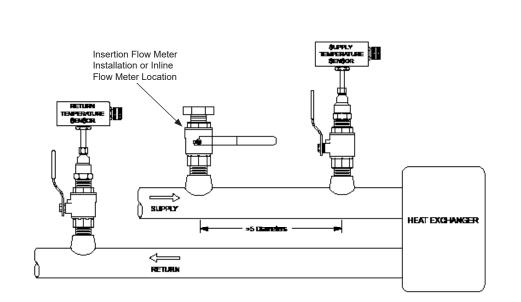
The supply and return sensors should be located in the piping system such that they only measure the temperature of the liquid flowing immediately in to and out of the section of the piping system where the energy measurement is made.
