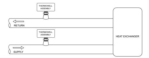
The supply and return sensors should be located in the piping system such that they only measure the temperature of the liquid flowing immediately in to and out of the section of the piping system where the energy measurement is made.
