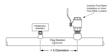
One sensor will be located in the same pipe with the flow meter. This sensor must be located at least 12" or 5 pipe diameters, whichever is greater, downstream from the flow meter.
