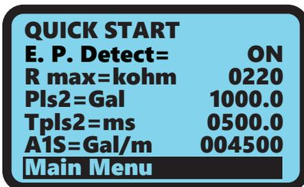
4. From Quick Start menu, push
