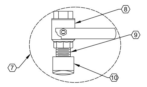
ONICON installation hardware kits consist of three separate component parts:
