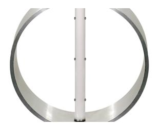
The FSM-3 utilizes a single, monolithic coil, designed to create a uniform magnetic field across the entire pipe, which is paramount for accurate flow measurement in installation locations with less than ideal flow profiles.
