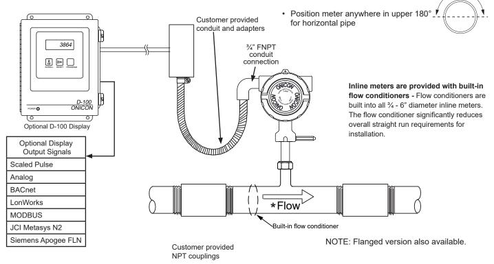
· Acceptable to install in vertical pipe
