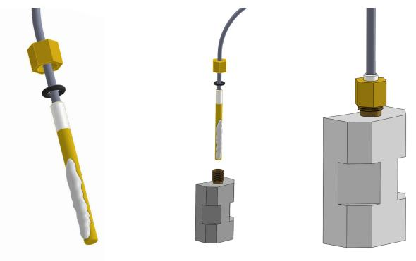
4. Apply thermal compound to the heat sink and install the clamp-on thermowell on to the pipe using the pipe strap as shown.
