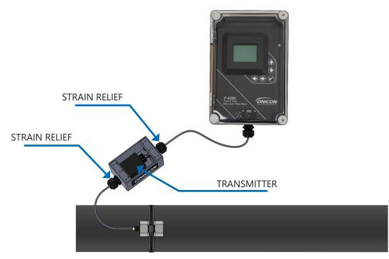
6. Tighten the strain reliefs and reinstall the junction box cover. Once the thermowells and sensors are fully installed and tested, insulate the thermowells and the pipe to complete the installation.
