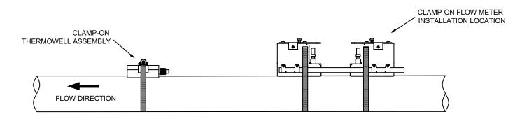
One temperature sensor thermowell will need to be placed in the same pipe as the mounting brackets. If it is an immersion thermowell, it must be located on the downstream side of the mounting brackets.
