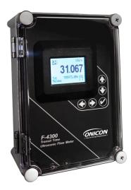
ONICON F-4000 Series Ultrasonic Flow Meters utilize the differential transit time method to measure the velocity of relatively clean liquids in full pipes. By measuring the difference between transit times of ultrasonic sound waves traveling between two transducers, the flow velocity and direction are accurately determined.
