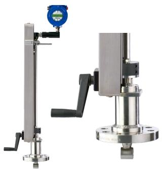
Insertion vortex flow meters detect the frequency of alternating low pressure vortices that are formed as flow is diverted around a bluff body. These swirling low pressure zones apply lateral pressure first to one side and then to the other of sensors located downstream of the bluff body. This causes the sensors to vibrate. The frequency of this vibration is directly proportional to the flow velocity.
