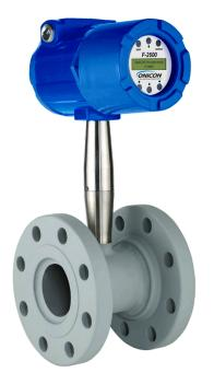
Vortex flow meters detect the frequency of alternating low pressure vortices that are formed as flow is diverted around a bluff body. These swirling low pressure zones apply lateral pressure first to one side and then to the other of sensors located downstream of the bluff body. This causes the sensors to vibrate. The frequency of this vibration is directly proportional to the flow velocity.
