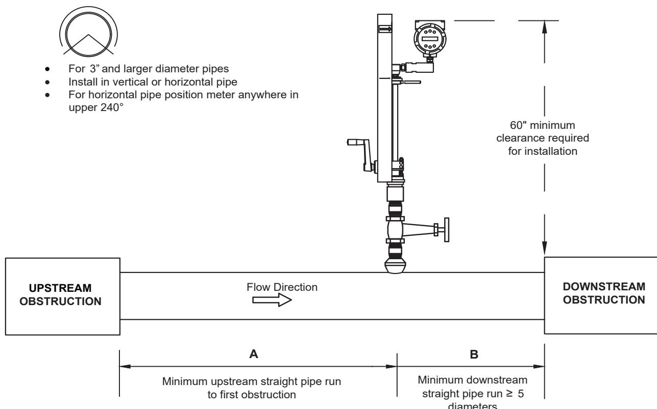
**NOTE: For liquid applications in vertical pipes, avoid installing with flow in the downward direction because the pipe may not be full at all points. Choose to install the meter with flow in the upward direction, if possible.**
