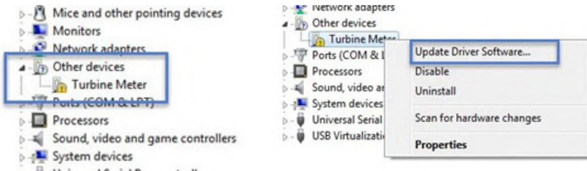
In the "Update Driver Software" screen, click "Browse..." and select the folder for the Configuration Tool which was provided by ONICON. Make sure the "Include Subfolders" check box is enabled and click "Next".
