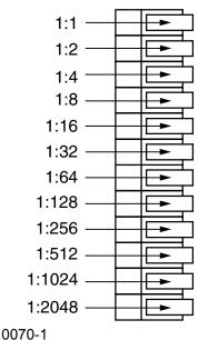
To set division ratio, turn ON each switch that is required to produce an arithmetic sum equal to the desired ratio. For example:
