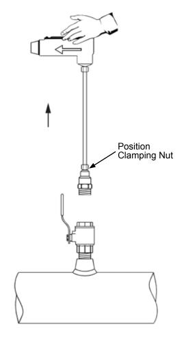
fully withdrawn. Usually a gentle twisting motion while withdrawing the meter will clear any obstruction and permit the meter to withdraw completely. (Excessive build-up on the stem may require the hot tap 'O' ring to be lubricated with silicone.)
