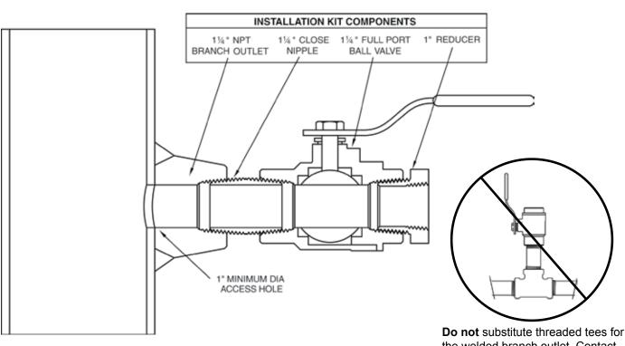
**Do not** substitute threaded tees for the welded branch outlet. Contact ONICON if you need installation hardware for threaded pipe.
