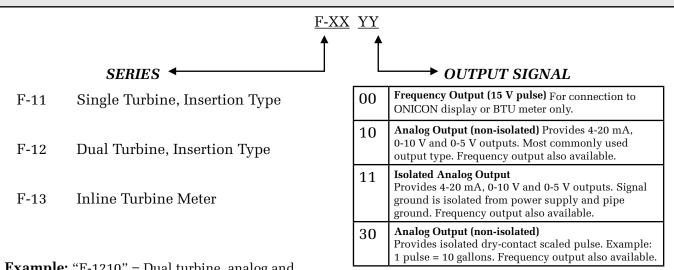
**Example:** "F-1210" = Dual turbine, analog and frequency outputs
