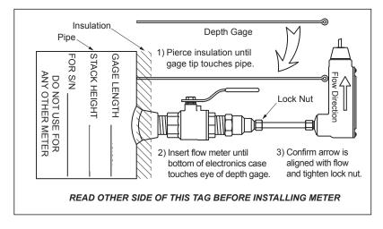
Prior to installing the meter, confirm that the stack height recorded on the tag is close to the actual stack height. Flow meter stems are intentionally over sized to allow for variations of at least 2" in the stack height. Contact ONICON prior to installation if there is any question regarding stack height or stem length. This will allow ONICON to offer you credit for your meter if you decide to exchange the meter for one with a different stem length. Returns may be subject to a restocking fee.
