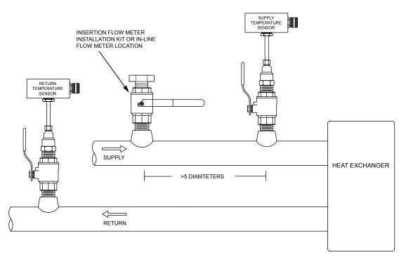
The supply and return sensors should be located in the piping system such that they only measure the temperature of the liquid flowing immediately in to and out of the section of the piping system where the energy measurement is made.
