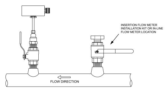
One sensor will be located in the same pipe with the flow meter. This sensor must be located at least 12" or 5 pipe diameters, whichever is greater, downstream from the flow meter.
