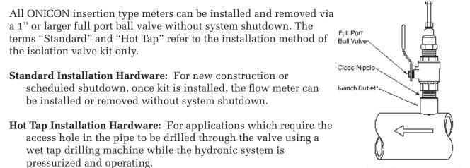
\*Weld-on filting, copper tee or saddle
