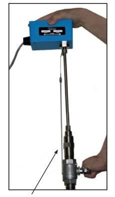
**Step 2:** Carefully withdraw the flow meter stem from the pipe until the sensor head is fully inside the hot tap adapter.
