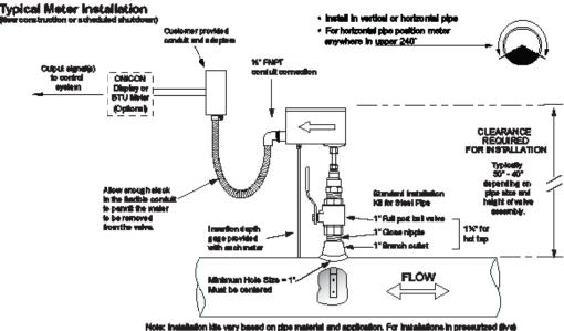
Nois: Insiallation kills vary based on pipe material and application. For installations in pressurized (if/ evelope, use "Hotizo" 11% inch installation kit and chill hole using a 1 inch wet iso chill.
