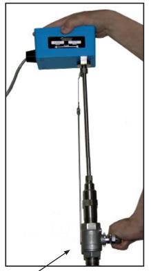
Step 3: After the meter is completely withdrawn, slowly close the valve to isolate flow.
