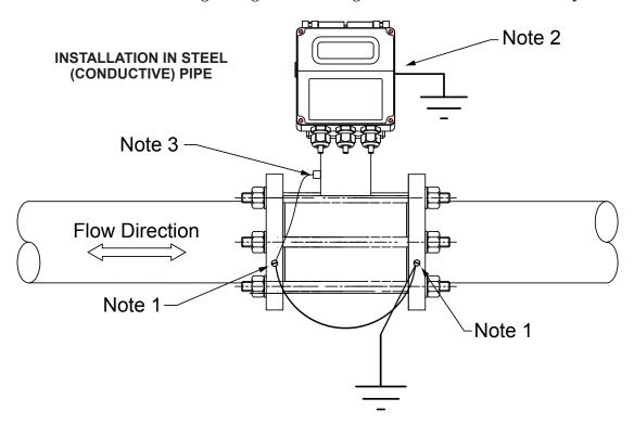
Note 1: Using a #21 (0.159") drill bit, drill a ½" deep hole in edge of each mating flange. Tap each hole using a 10-32 tap. Secure the included ring connectors and grounding wires to the flange using the provided green grounding screws. (Alternate method: Weld 10-32 studs not provided to the flange edges and attach ring connectors with 10-32 nuts not provided.)
