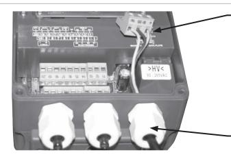
Step 6: Wire the connector as shown based on input type. Earth connection must be made.
