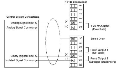
Typical Connections For Bi-Directional Flow and No ONICON Peripheral Device
