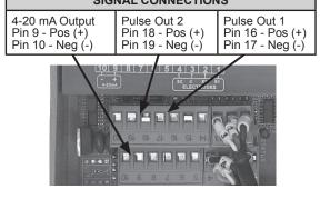
Typical Connections With No ONICON Peripheral Device
