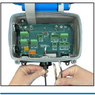
When connecting the cable to the transmitter, feed one sensor cable (out of the three) through the conduit adapter/ strain relief at a time. Once all three cables are through the connector, tighten the internal/ strain relief cable grip.
