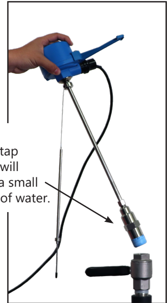
Step 4: After the valve is completely closed, unscrew the hot tap adapter from the valve. For hot water meters, partially unscrew the adapter to vent pressure before fully removing the meter.
