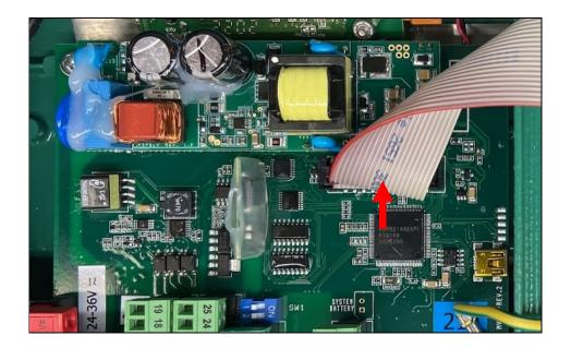
5. Once all connections are detached, remove the four Phillips screws (note ground wire on the lower right screw for reassembly).
