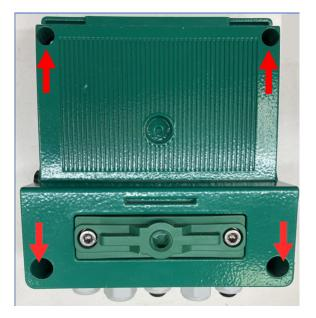
3. Carefully detach the front panel, (note ribbon cable connection).
