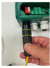
Loosen the barrel cover to expose the RJ-45 coupler. (Again, do not allow the coupler to rotate).
