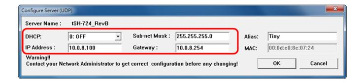
11. Change your network settings including IP, Mask, and Gateway (if used). **Warning: Changing network settings can cause network connectivity issues and should be done with caution.**
