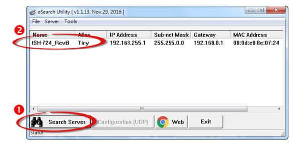
10. Once you have the IP information of the module, you can change your computer's network settings parameter to match those of the MODBUS TCP/IP module, or you can click on the Configuration (UDP) button to alter the module's network settings. Clicking on Configuration (UDP) will display the following window. **Note: Consult your Network Administrator to get the correct configuration before making any changes.**
