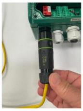
A. Loosen the strain relief nut completely and slide down the existing cable (if applicable).
