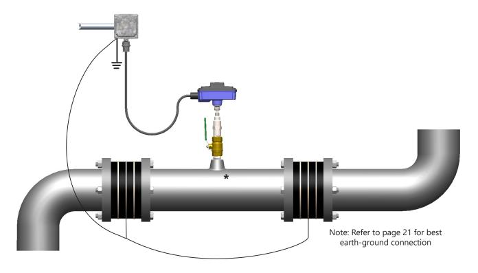
\* Additional straight run may be required upstream of the upstream grounding ring based on the nature of the upstream obstruction. Refer to the chart in Section 3.1 on page 8 of this manual to determine how much straight run is required.
