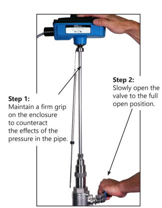
**Step 4:**Orient the enclosure to parallel with the pipe and in alignment with the flow direction arrow.
