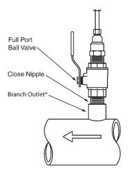
\*Weld-on fitting, copper tee or saddle
