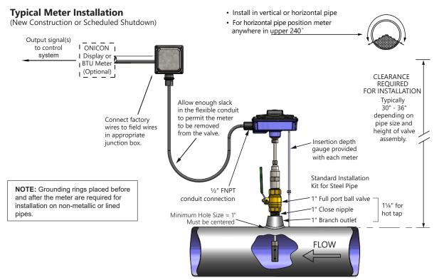
Note: Installation kits vary based on pipe material and application. For installations in pressurized (live) systems, use "Hot tap" 11/4 inch installation kit and drill hole using a 1 inch wet tap drill.
