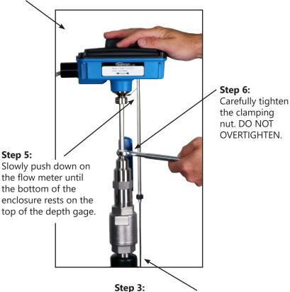
Use the end of the depth gage to pierce any insulation that may be present and rest the gage on the outside wall of the pipe.
