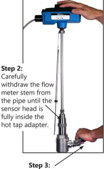
After the meter is completely withdrawn, slowly close the valve to isolate flow.
