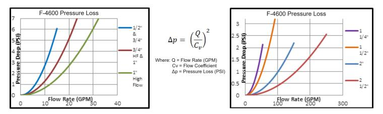
\*ONICON defines the "design" flow rate as the maximum continuous flow expected by the application under normal operating conditions. The pressure drop for the ONICON design flow rates is  $\leq 1.7$  psi.
