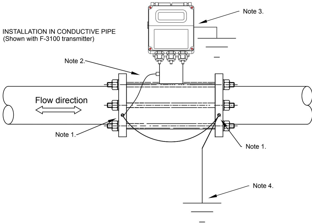
**Note 1.** Using a #21 (0.159") drill bit, drill a 1/2" deep hole in edge of each mating flange. Tap each hole using a 10-32 tap. Secure the ring connectors (provided) and grounding wires to the flange using the green grounding screws (provided).
