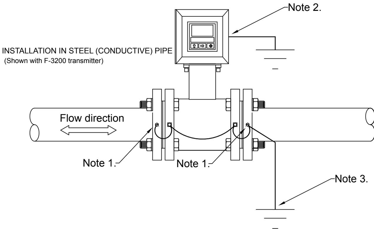
**Note 1.** Using a #21 (0.159") drill bit, drill a 1/2" deep hole in edge of each mating flange. Tap each hole using a 10-32 tap. Secure the ring connectors (provided) and grounding wires to the flange using the green grounding screws (provided).
