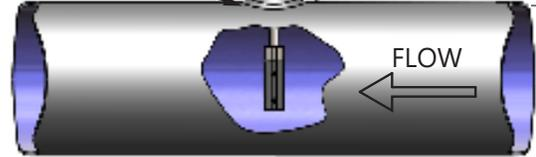
Note: Installation kits vary based on pipe material and application. For installations in pressurized (live) systems, use "Hot tap" 1/4 inch installation kit and drill hole using a 1 inch wet tap drill.
