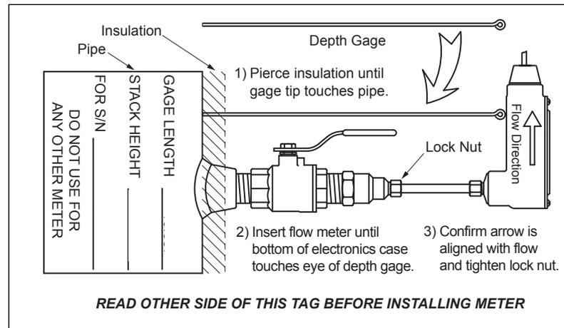
Prior to installing the meter, confirm that the stack height recorded on the tag is close to the actual stack height. Flow meter stems are intentionally over sized to allow for variations of at least 2" in the stack height. Contact ONICON prior to installation if there is any question regarding stack height or stem length. This will allow ONICON to offer you credit for your meter if you decide to exchange the meter for one with a different stem length. Returns may be subject to a restocking fee.
