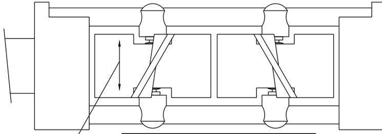
Turbines must be free to slide back and forth on the shaft with at least .015" of movement.
