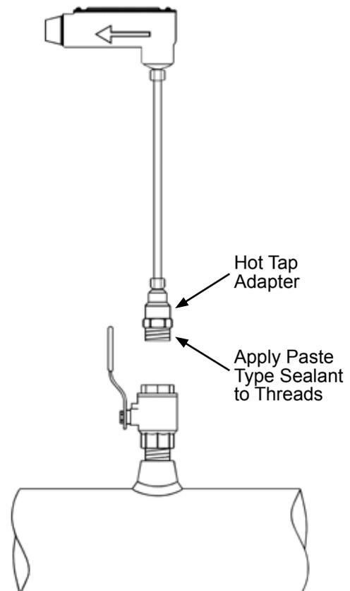
1. Open valve completely, loosen the position clamping nut, and insert the meter until the bottom of the electronics case touches the eye of the depth gage. (Pierce insulation with gage until the tip touches the pipe.)
