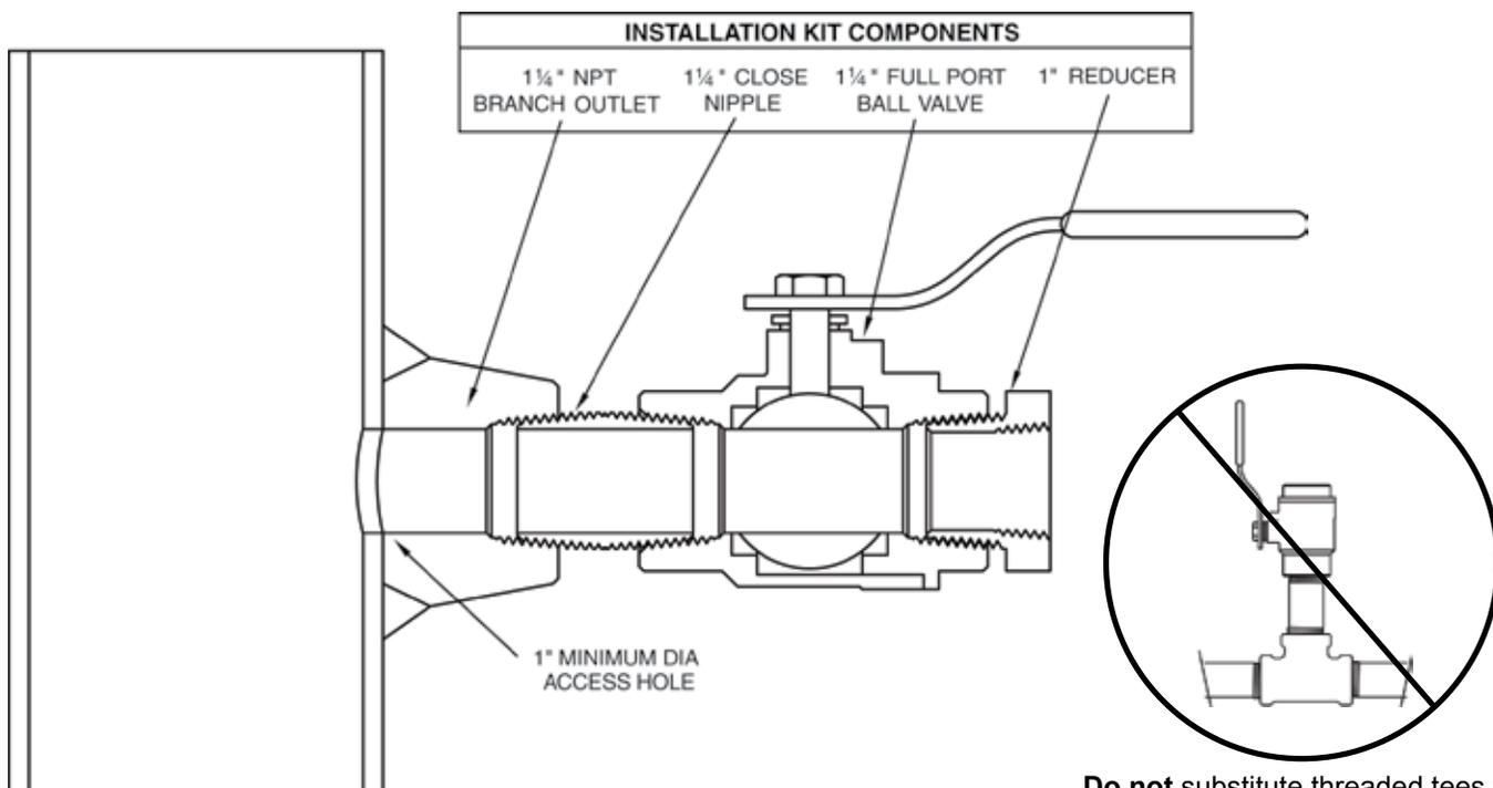
**Do not** substitute threaded tees for the welded branch outlet. Contact ONICON if you need installation hardware for threaded pipe.
