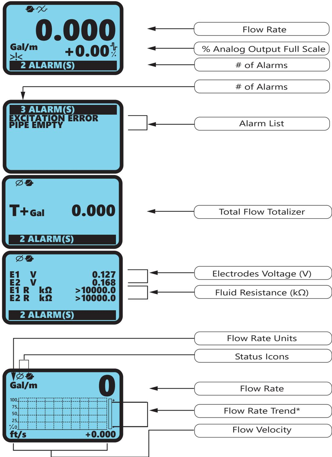
\* Trend is a graph of the % of analog output full scale over the last 100 seconds.
