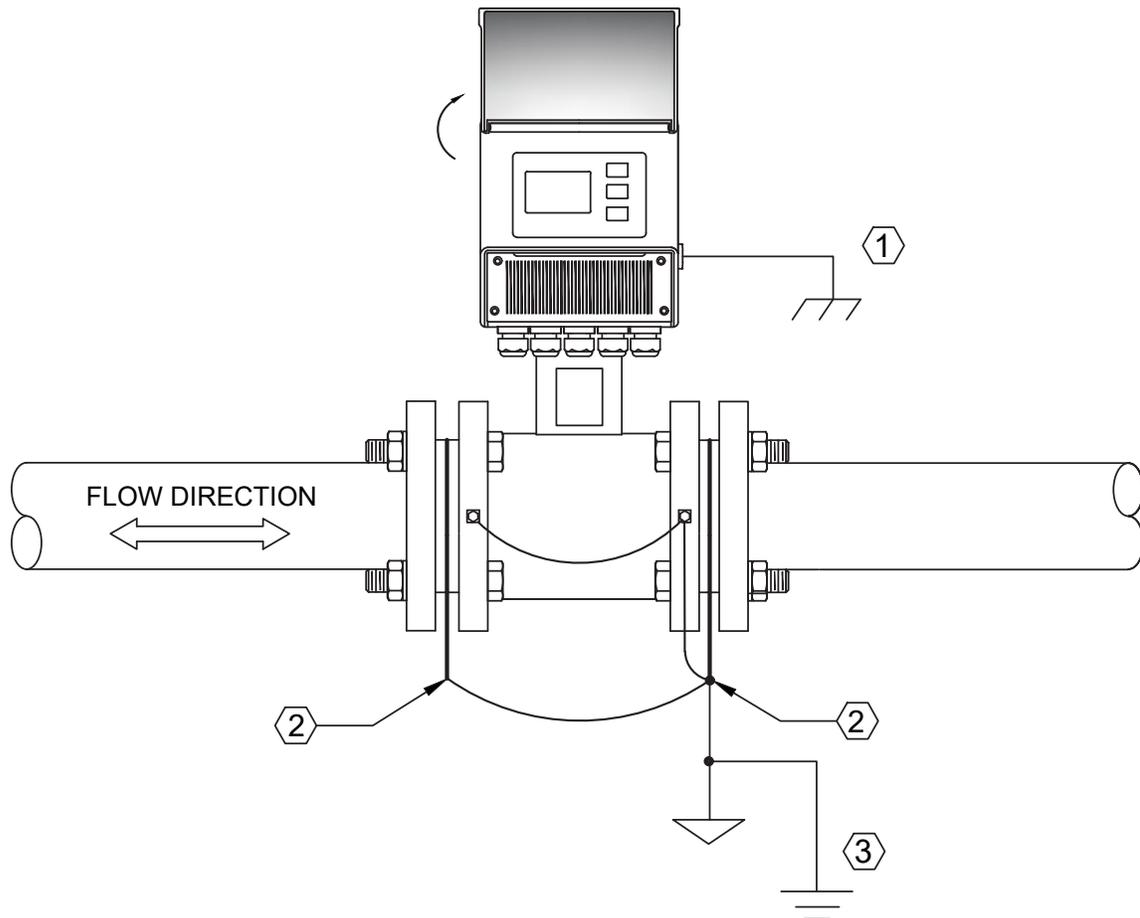
1. Provide a protection ground connection at the input power terminals inside the transmitter enclosure
