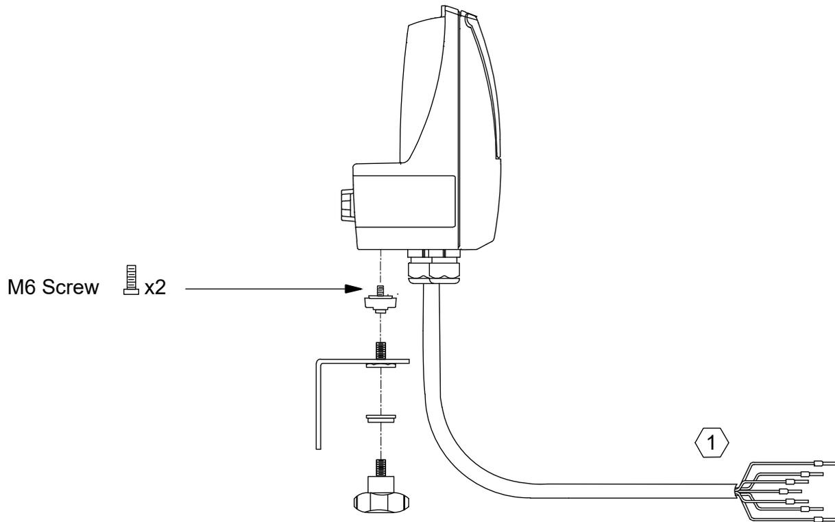
1. Cable wires are labeled with numbers. Refer to 3.3.5 Remote Mount Cable Wiring Connections for more details.
