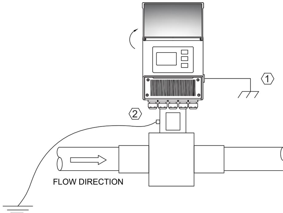
1. Provide a protection ground connection at the input power terminals inside the transmitter enclosure
