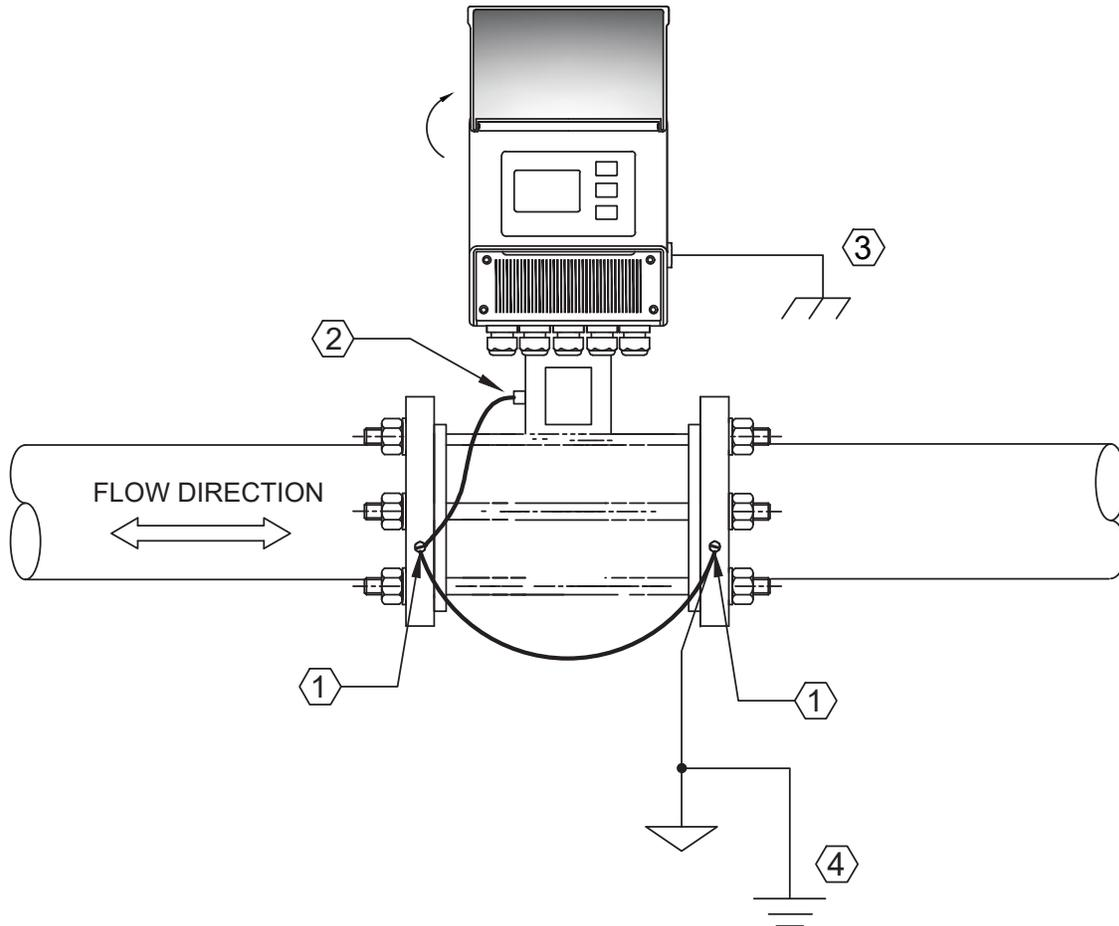
1. Using a #21 (0.159") drill bit, drill a 1/2" deep hole in edge of each mating flange. Tap each hole using 32 tap. Secure the ring connectors (provided) and grounding wires to the flange using the green grounding screws (provided).
