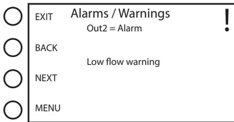
**Alarms / Warnings** provides the user with real time operating information. Warning messages alert the user to potential problems. Warnings are indicated by an exclamation point (!) in the upper right-hand corner of the display.
