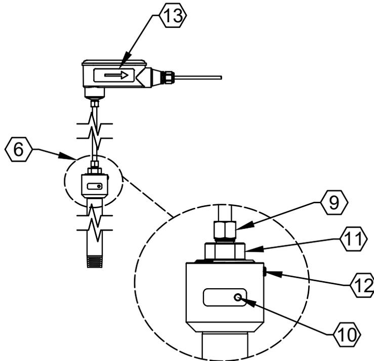
**6. (Hot Tap Adapter) Preload Housing****9. Stem Locking Collet Nut**
