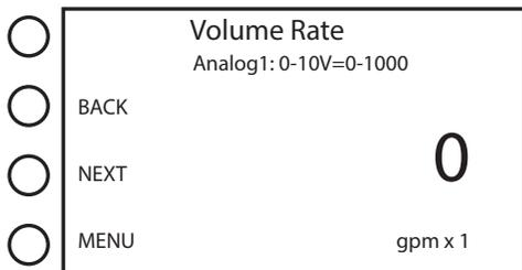
**Volume Rate** provides a continuous display of the instantaneous flow rate from the meter. Scaling for the 4-20mA and 0-5V/0-10V analog outputs will also be displayed on this page.
