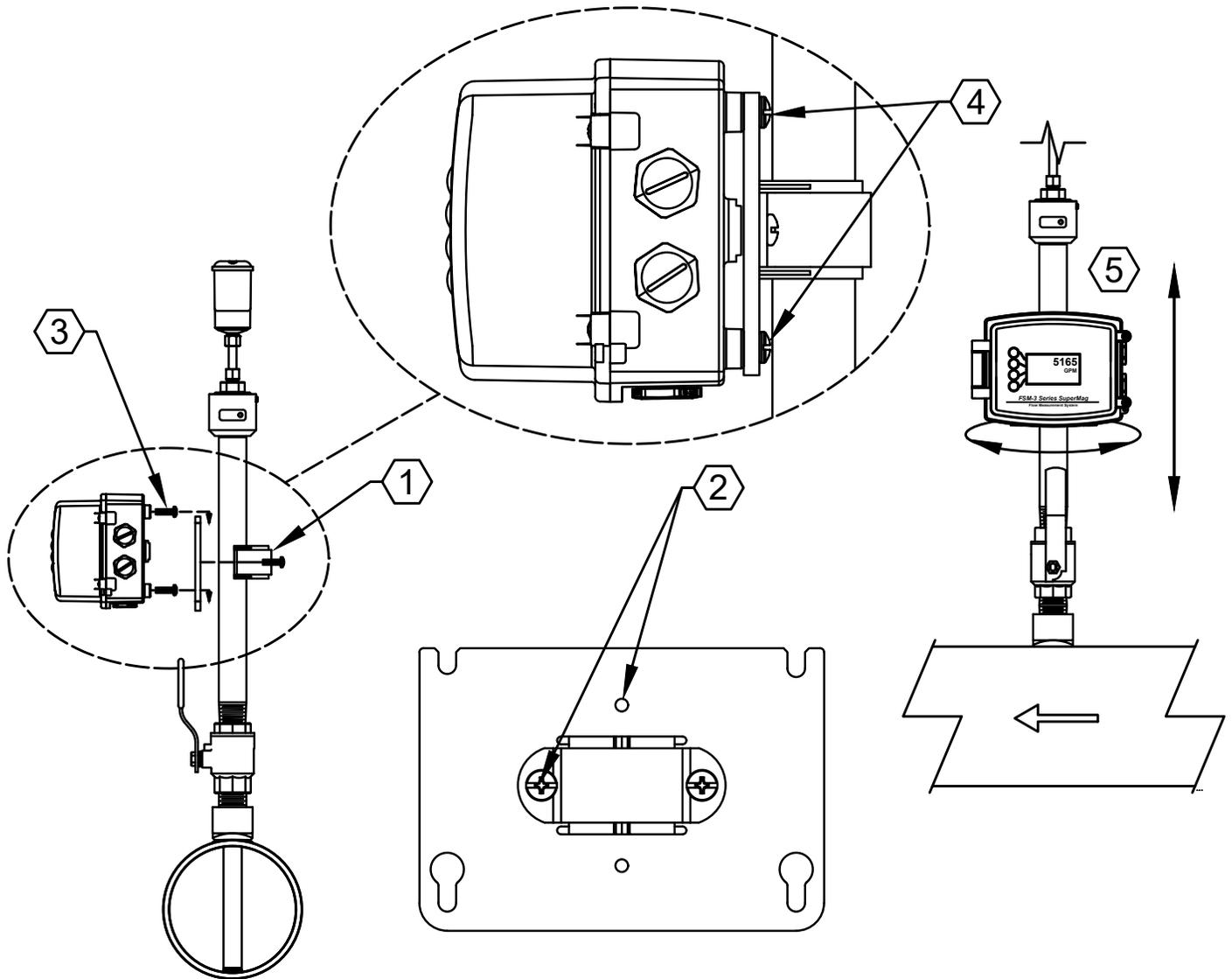
1. Install the integral mounting bracket on the hot tap adapter fitting as shown
