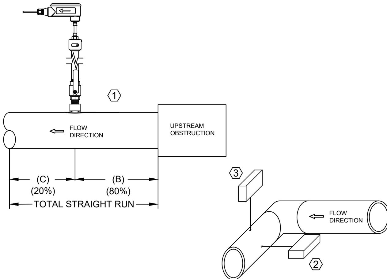
1. Install the flow meter in a section of pipe with the longest un-obstructed straight run available. If the published straight run recommendations cannot be met, locate the flow meter with 80% of the available straight run upstream
