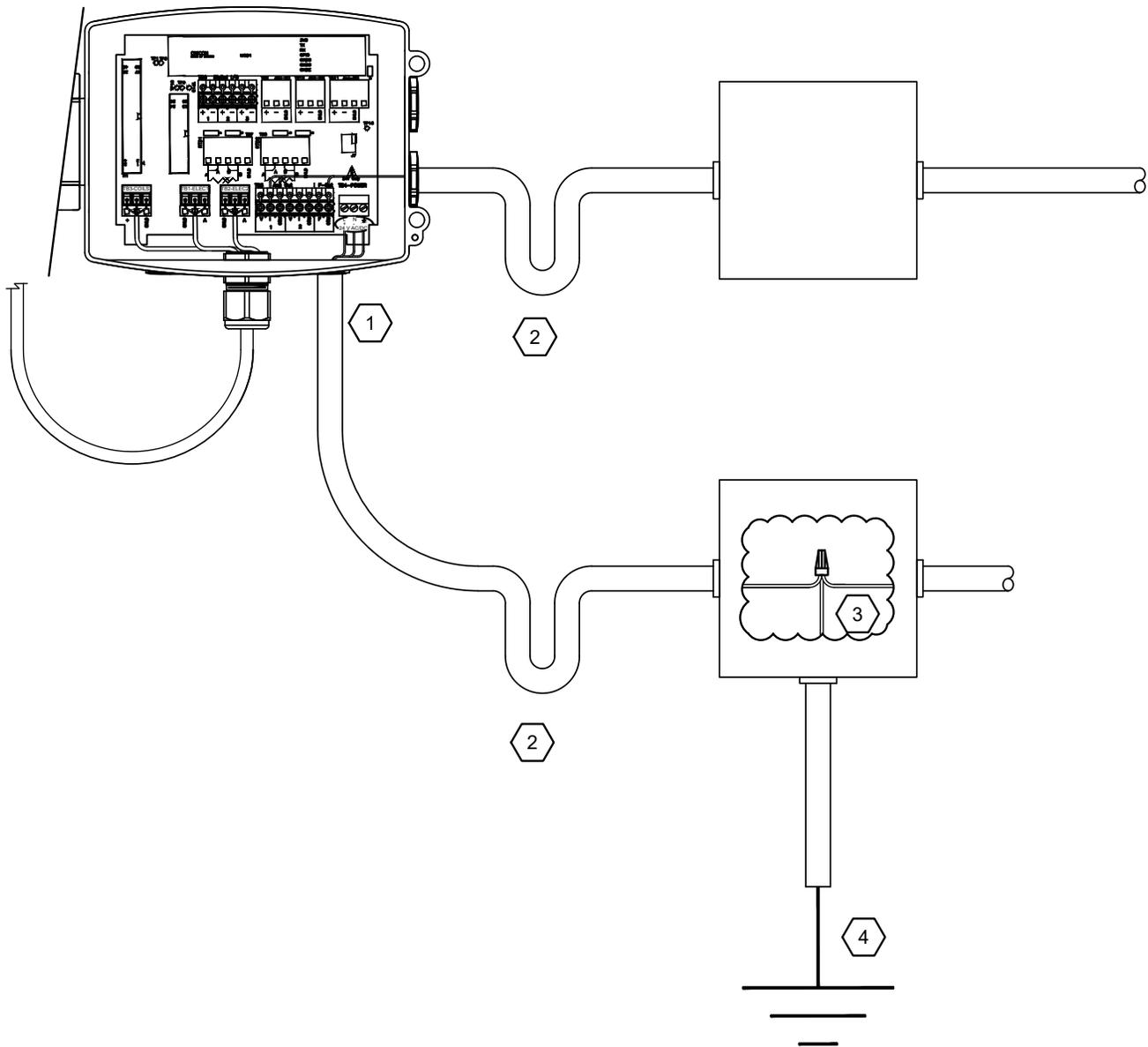
1. Route input power and ground wires through separate conduits and junction boxes from other signal wires
