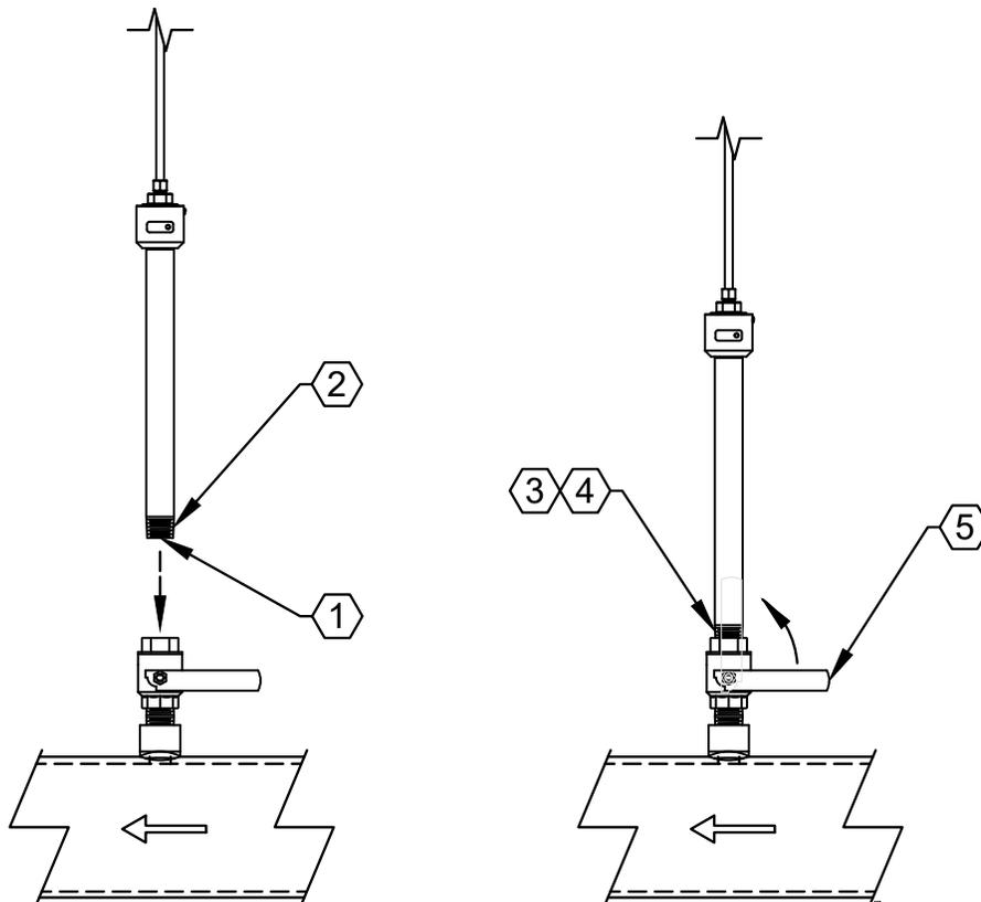
1. Fully retract the flow sensor into the hot tap adapter fitting
