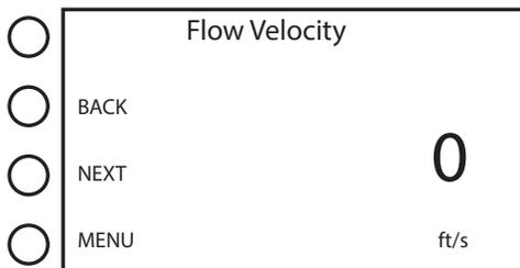
**Flow Velocity** provides a continuous display of instantaneous velocity from the meter.
