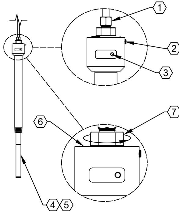
1. Use a  $\frac{5}{8}$ " open end wrench to loosen the stem locking collet nut
