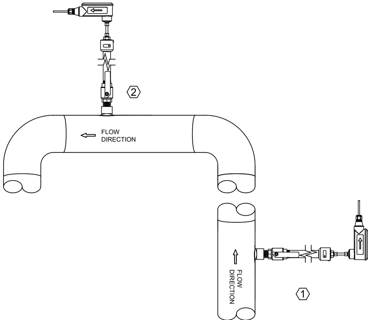
1. Installation of the FSM-3 flow meter in vertical pipes is acceptable. Flow in the upward direction is recommended in non-pressurized (open loop) systems
