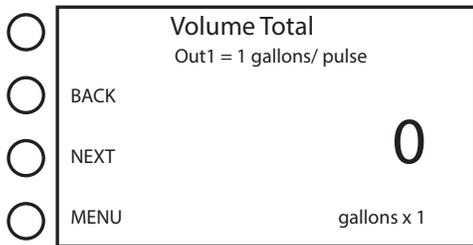
**Volume Total** is a non-resettable flow total. It can only be reset when the meter is recalibrated. It will roll over to zero when the maximum total has been accumulated. If one of the three digital outputs have been configured to totalize flow, the output and pulse scaling will be displayed on this page.
