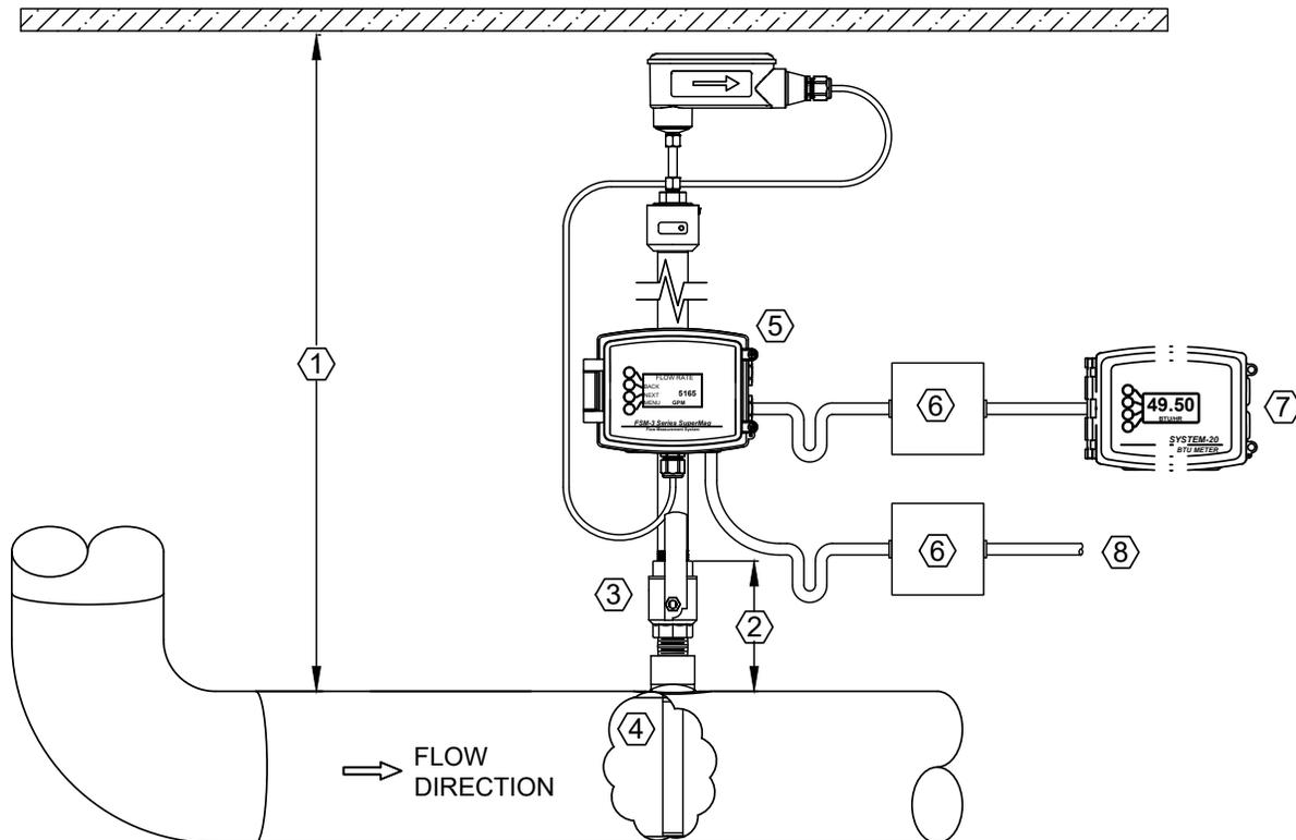
1. Prior to locating the flow meter installation kit, review the Overhead Clearance and Installation Details diagram in Section 3.1.1
