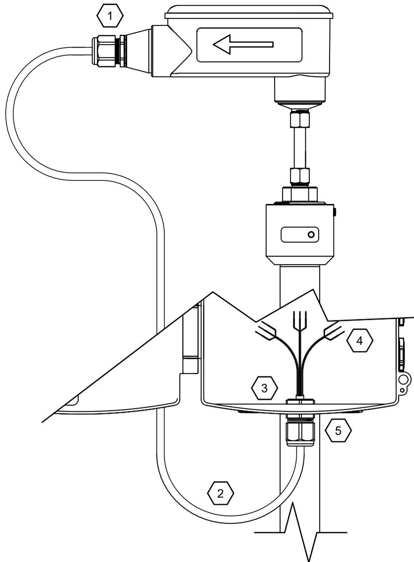
1. Electrode and coil wires are pre-attached via pluggable terminal blocks inside the flow sensor enclosure
