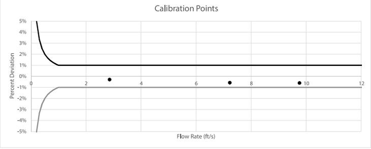
ONICON Incorporated certifies that this flow meter was calibrated against standards accurate to 0.1% and traceable to the National Institute of Standards and Technology (N.I.S.T.).
