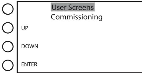
Momentarily press ENTER to access the operating mode (User Screens) display pages shown here. Next, verify that the meter is functional by stepping through the pages and confirming the flow rate and velocity are within expected norms.
