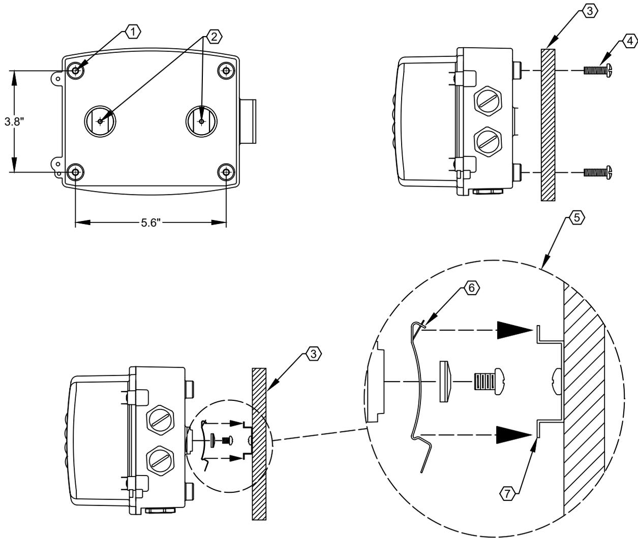
1. Threaded wall mounting hole locations, 1/4" -20 UNC thread, 1/2" depth, four (4) places. Refer to appendix for hole drilling template
