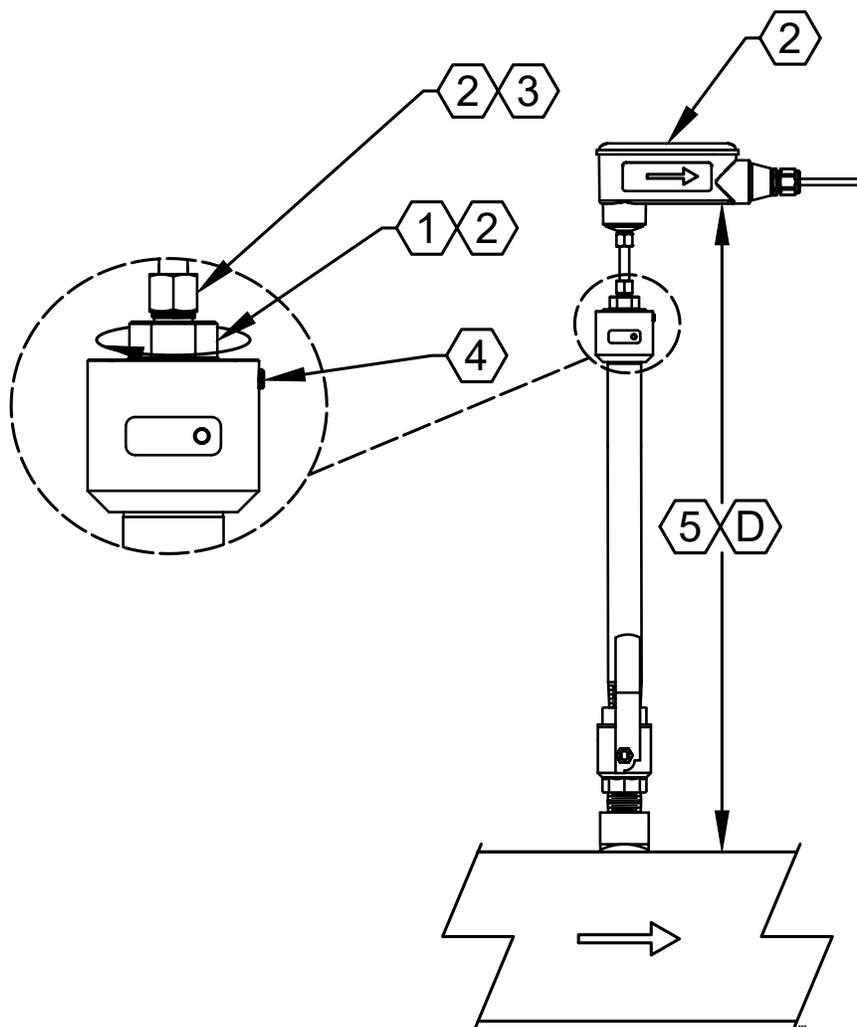
1. Use a 1" open end or crescent wrench to tighten the preload fitting. The preload fitting will be flush with the hot tap adapter preload housing when complete, approximately 1.25 turns clockwise
