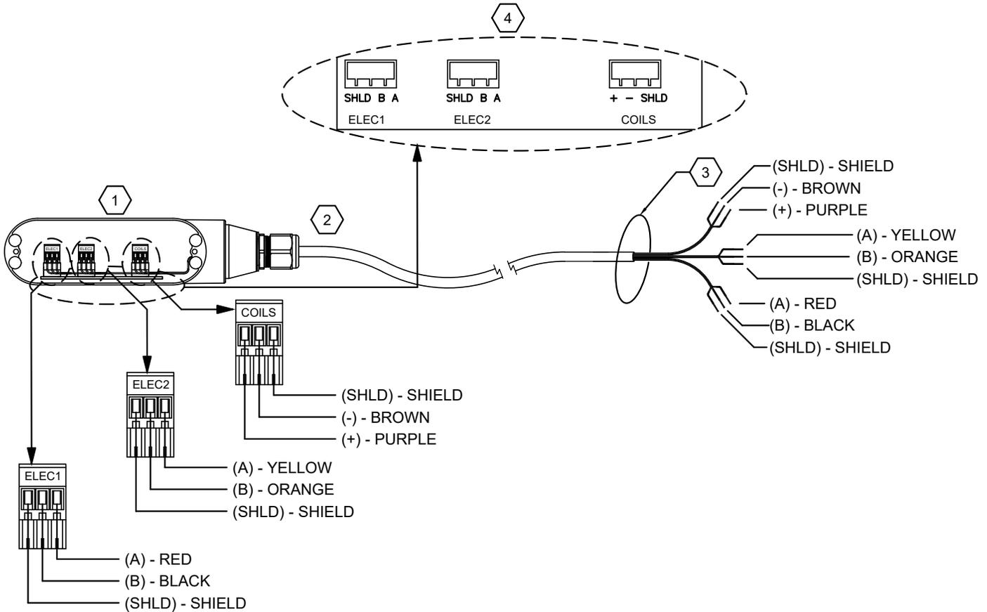
1. Remove flow sensor enclosure cover to gain access to coil and electrode wire terminal blocks
