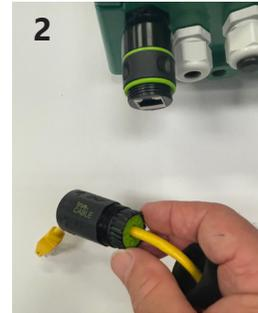
1. When ready to connect the TCP/IP network, first thread the nut, then slip the green cable seal over the cable, then the connection cover as shown.
