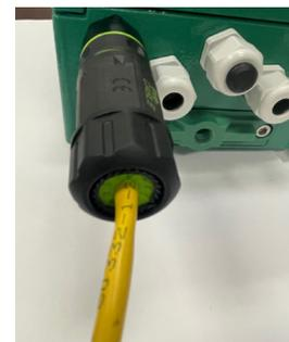
3. Connect the field cable to the RJ-45 coupler, then carefully thread the connection cover on the coupler until it is finger tight against the green o-ring. Use caution to avoid twisting the cable.
